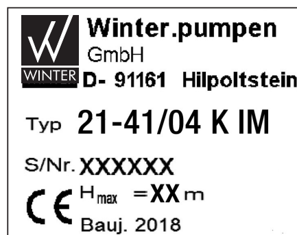
Illustration 4 Example of a name plate on the pump
